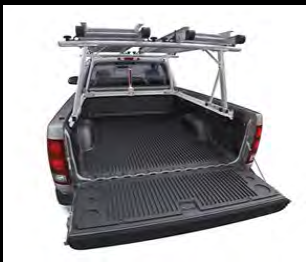
Overhead utility rack 226kg capacity
