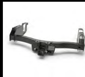
Genuine GM heavy duty towbar - rated 5000kg
