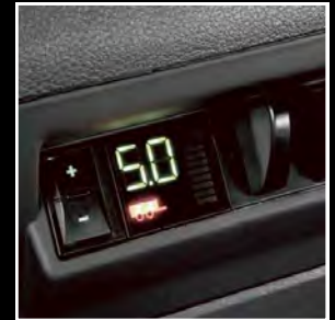
Integrated trailer brake module
